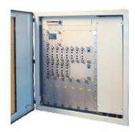
Central Battery System, shortly Central Battery is characterized by this, that all emergency luminaires are supplied from one source. It is only adapted to one nominal voltage ie 230VAC/3x230VAC.
